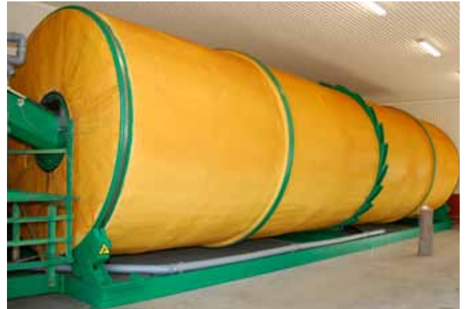
The drum is fully enclosed, to control the process
