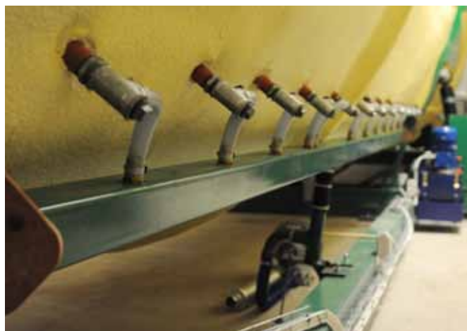
Air is blown into the compost by a fan
