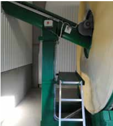
Feeding and discharge are to/from the center of the drum. The inside of the drum is covered by layers of a special color to withstand corrosion
