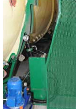
Rotation is powered by efficient hydraulics
