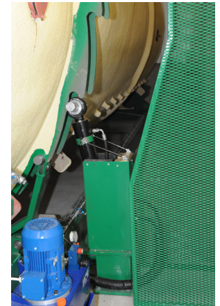
Rotation is powered by efficient hydraulics
