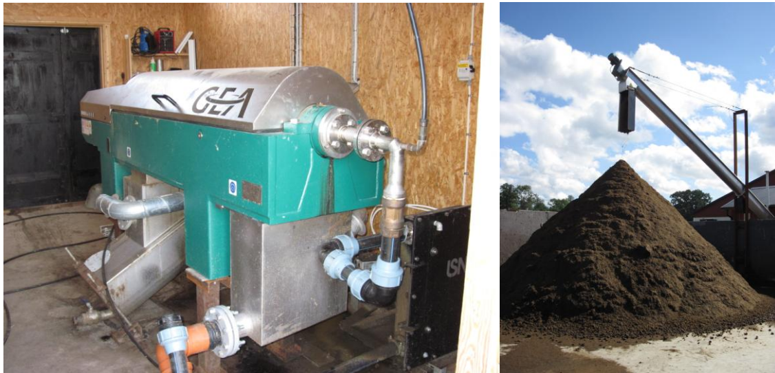
Figure 26. GEA centrifuge decanter manure separator ( www.westfalia-separator.com ).
