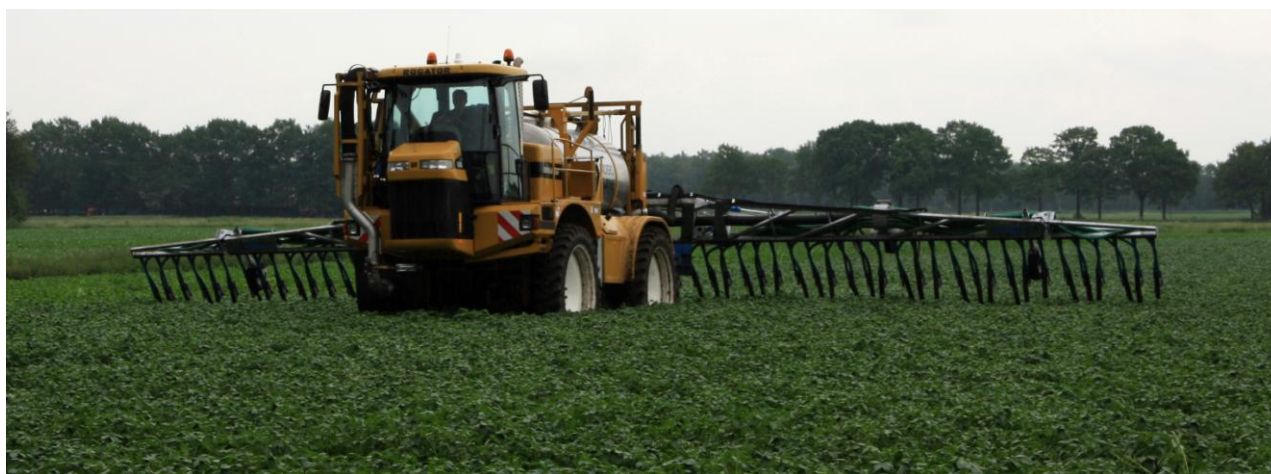
Figure 11. A RoGator slurry spreader with a boom with trailing shoes. The spreader was modified by Kumac specifically for spreading reverse osmosis concentrate.
