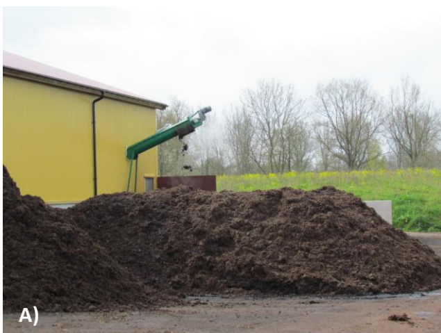
Figure 23. a) Output screw conveyor for compost from the drum and b) loading the finished compost on a trailer for transport to the packaging facility.
