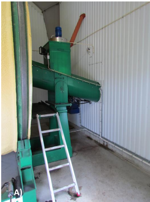
Figure 22. a) The input screw conveyor for substrate loading into the composteur drum as seen from inside the building and b) temperature sensors in the drum composteur.
