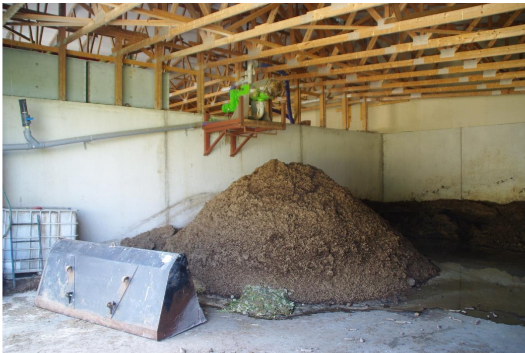
Figure 24. The Bauer screw press separator mounted above the solid fraction collection pad.
