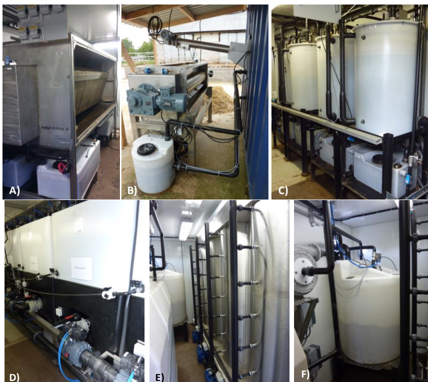
Figure 3. a) Coarse 200 \mu\text{m} filter (rotating square sieve) for incoming slurry, with filtrate collection tanks underneath, b) drum press for solid fraction, c) parallel fine mesh filters at 50 \mu\text{m} with filtrate collection tanks underneath, d) parallel struvite precipitation tanks, e) ammonia strippers, and f) acid scrubber unit.
