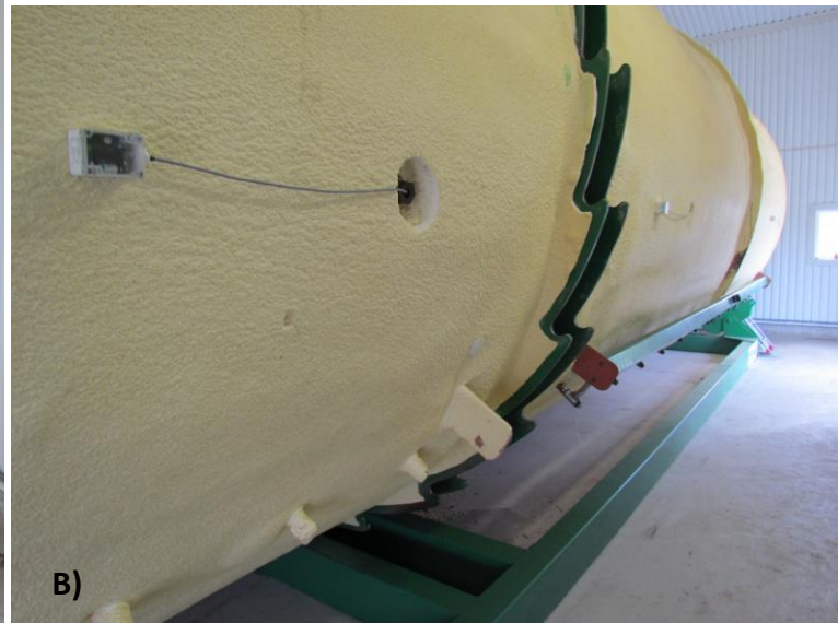
Figure 22. a) The input screw conveyor for substrate loading into the composteur drum as seen from inside the building and b) temperature sensors in the drum composteur.
