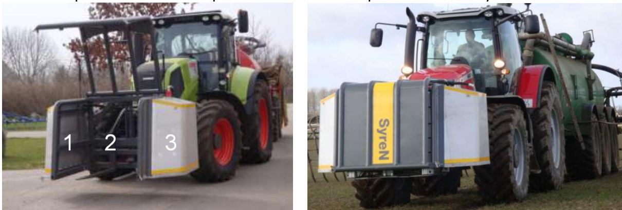
Figure 17. The SyreN-system includes three tanks installed on the front of the tractor. 1) Tank for iron sulphate, 2) site of tank for sulphuric acid, and 3) tank for water for cleaning the system.
