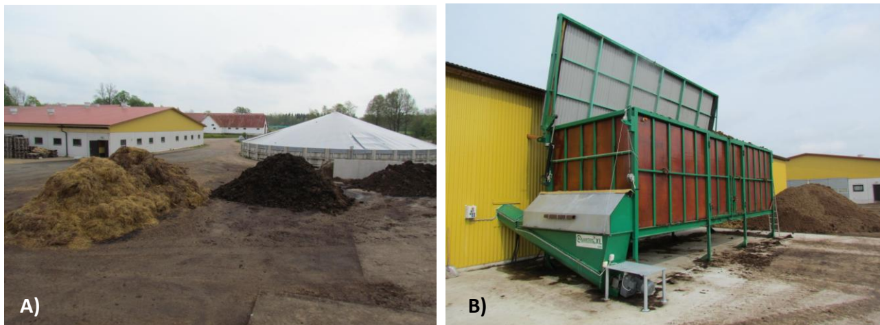
Figure 21. a) Hard standings and manure pad used for receiving and mixing solid manure from cows, horses and pigs and the separated manure solids from slurry and b) the loading container and input screw conveyor for substrate loading into the composter.
