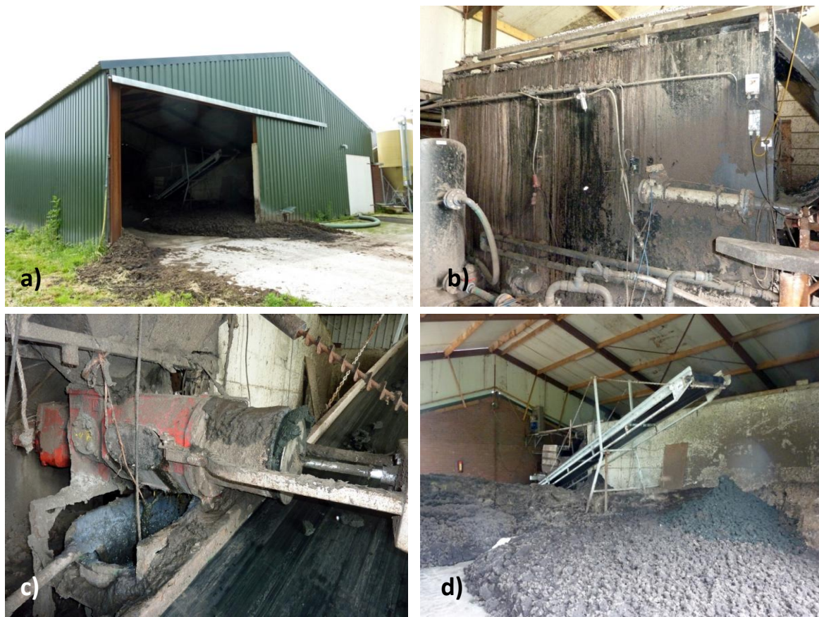
Figure 9. a) Manure processing shed, b) polymer mixing tank on far left in front of large flotation tank, c) screw press separator with conveyor for transport of solid fraction to (d) covered storage.
