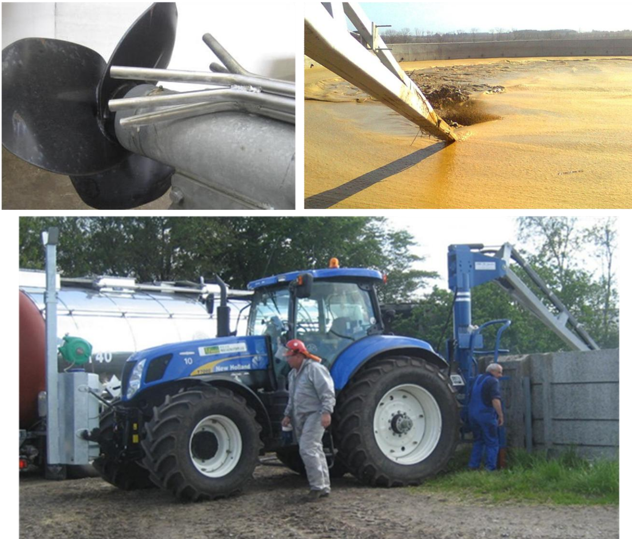
Figure 14. Ørum TF-12 slurry acidification system (Photo: Ørumsmeden A/S). Top left, acid injectors mounted onto a Ørum GMD slurry mixer. Top right, mixing and acidification process. Bottom, Ørum TF-12 rear mounted a tractor with a safety shower and water tank mounted on the front. The sulphuric acid tanker truck is behind the tractor.
